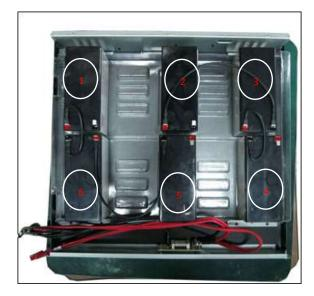
Please connect BAT1+ and BAT6- with black wiring Please connect BAT6+ and BAT5- with black wiring Please connect BAT2+ and BAT3- with black wiring Please connect BAT3+ and BAT4- with black wiring
