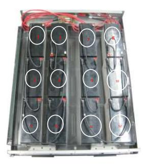
Please connect BAT1-and BAT3+ with black wiring Please connect BAT3-and BAT5+ with black wiring Please connect BAT5- and BAT6+ with black wiring Please connect BAT6- and BAT4+with black wiring Please connect BAT4- and BAT2+with black wiring Please connect BAT7-and BAT9+ with black wiring
