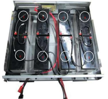
Please connect BAT7+and BAT8- with black wiring Please connect BAT8+ and BAT1- with black wiring Please connect BAT1+ and BAT2- with black wiring Please connect BAT3- and BAT4+with black wiring Please connect BAT4- and BAT5+with black wiring Please connect BAT5- and BAT6+with black wiring Please connect BAT7- , BAT6- and output with long black wiring
