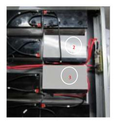
Please connect BAT2+ and FUSE with red wiringPlease connect BAT3+ and FUSE with red wiringPlease fix batteries into the battery case`s connect as below
