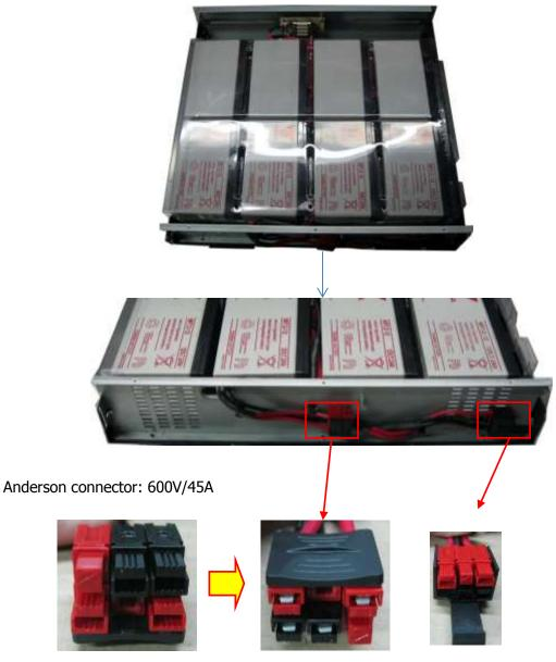
Battery Wiring of PowerWalker VFI 3000 RT LCD Battery Pack 1. Please assemble 12pcs batteries into the Battery Case`s and connect batteries with wires as below:
