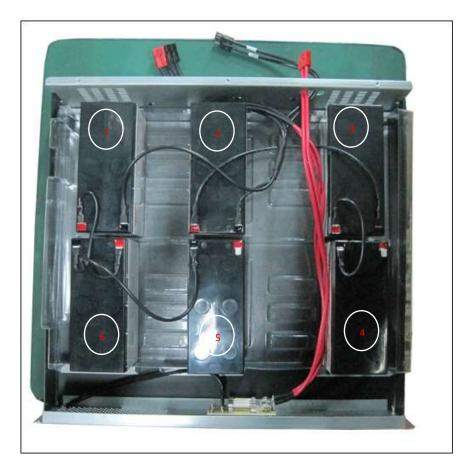
Please connect BAT5+ and FUSE with black wiring Please connect BAT4+ and FUSE with black wiring Please connect BAT1- , BAT2- and output with long black wiring
