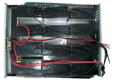
Please connect BAT1+ and FUSE with red wiring Please connect BAT7+ and FUSE with red wiring Please connect BAT2-, BAT8- and output with long black wiring 2. Please fix batteries into the battery case`s connect as below
